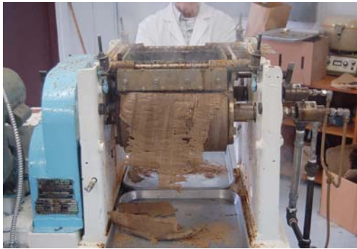
Drying high protein salmon concentrate on double drum dryer
